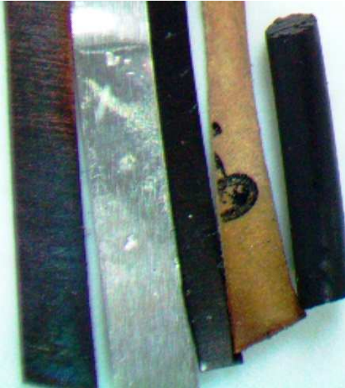
R-404A Control: Cu, Al, Fe, Gasket, O-Ring
