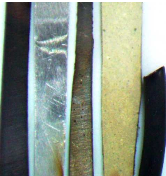
R-134a Control: Cu, Al, Fe, Gasket, O-Ring
