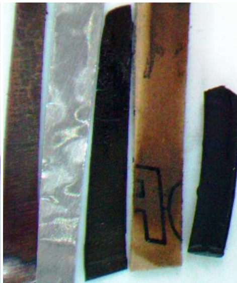
R-407C Test: Cu, Al, Fe, Gasket, O-Ring
