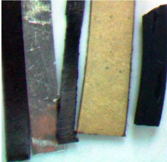
R-404A Test: Cu, Al, Fe, Gasket, O-Ring
